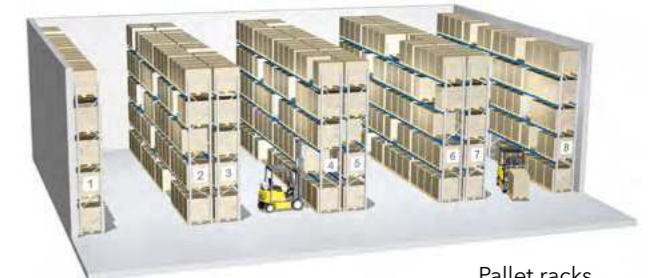
Pallet racks in conventional arrangement
