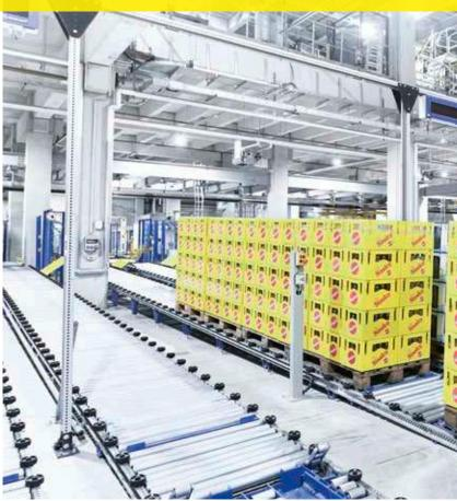
For special requirements SSI SCHAEFER has also developed a new type of inspection system for fully automated empties detection based on its WAMAS® Vision software, programmed special algorithms for the control software, and tailored the features of the HBW. Background: The empties pallets returned from retailers to the logistics center consist mainly of a mix of products and bottle sizes. However, the production systems fill by product. The installed empties management for
