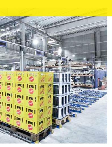
the degree in which the empties are mixed and the needs of the production lines, controls their further transport. The needs-based supply of filling lines with empties is a central function of the new logistics system.
