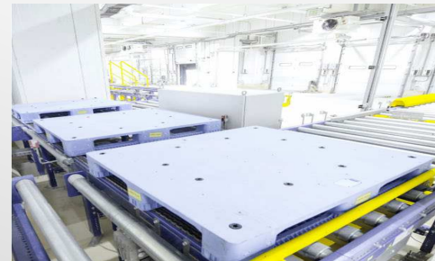
Food products are carried by forklifts to the infeed conveyor
