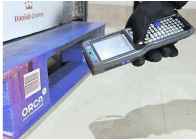
Tagging of pallets using QR codes for real-time monitoring
