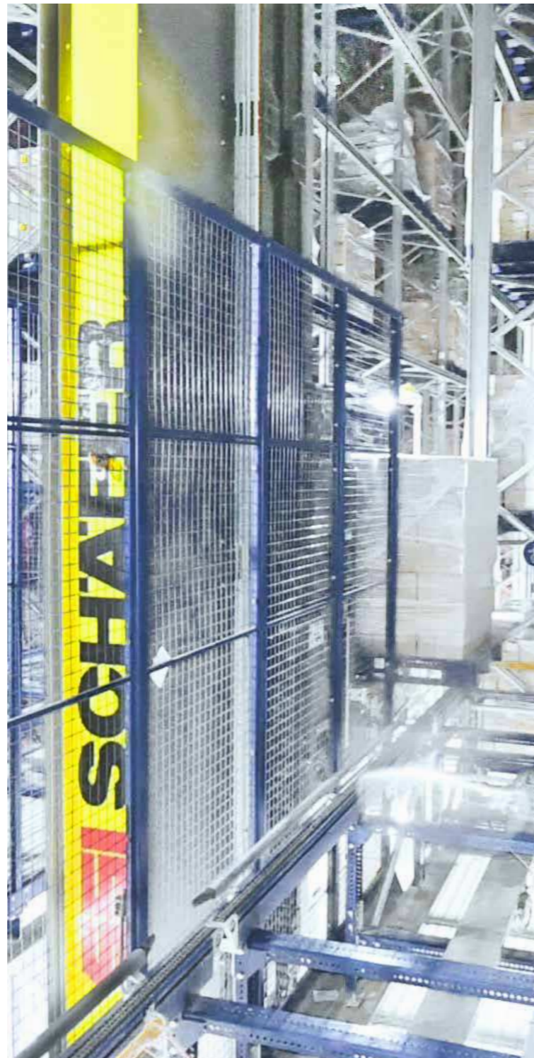
SSI Exyz stores and retrieves pallets
