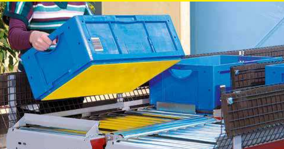
▲ Specially coated base of totes for the low noise conveying system ▼ Short distances between A-Frame and replenishment rack
