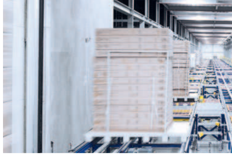
Powerful conveying system for Euro pallets and big box steel pallets
