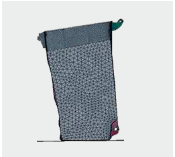
Computer simulation of drop test
