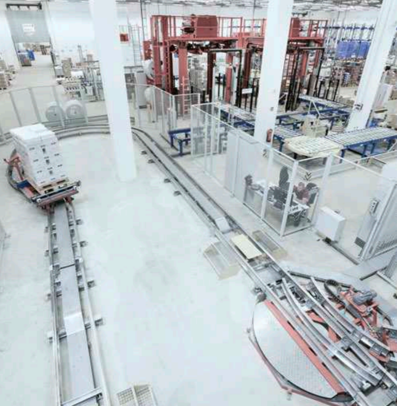
Transport between points of demand via a rail guided vehicle system
