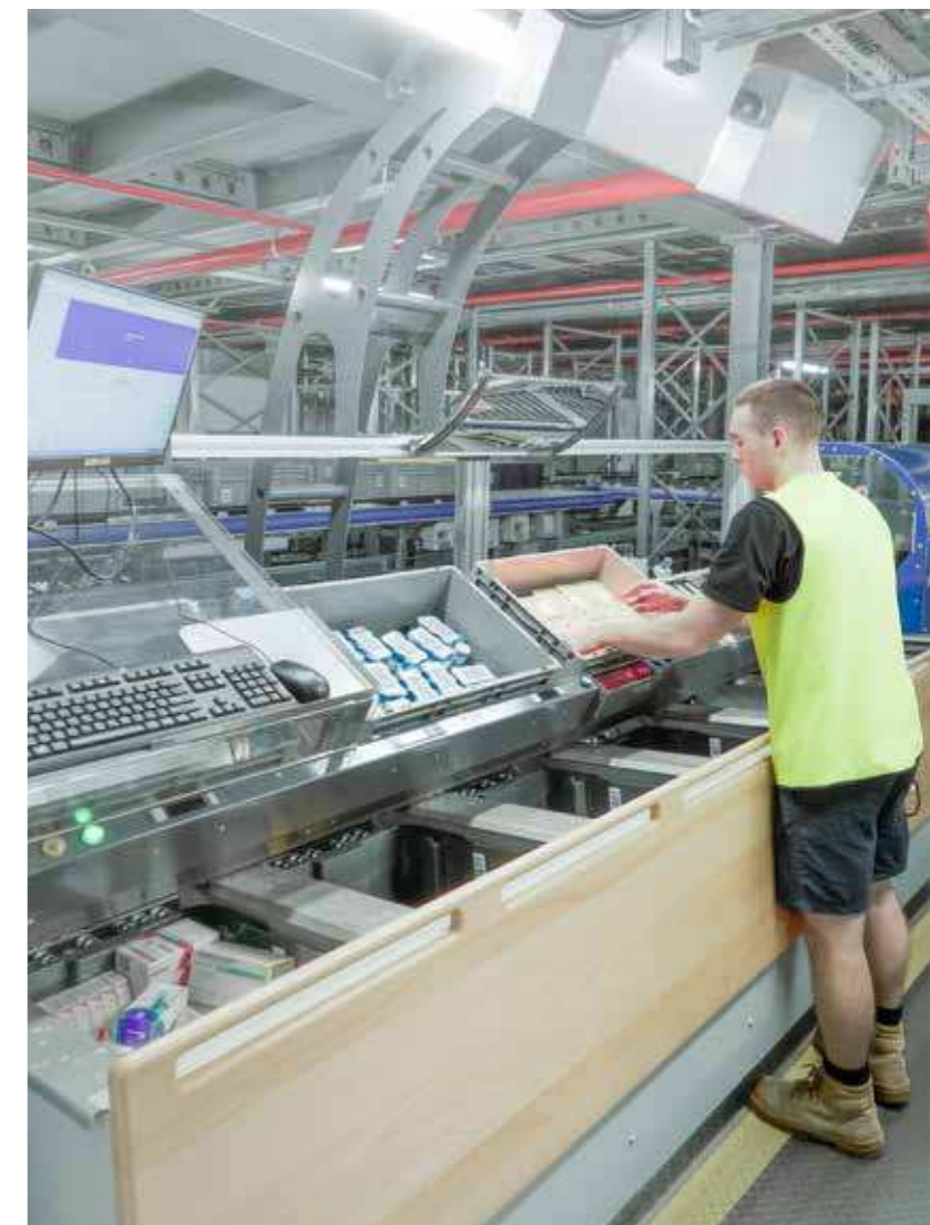
Ergonomically-optimized goods-to-person two-level Advanced Pick Stations
