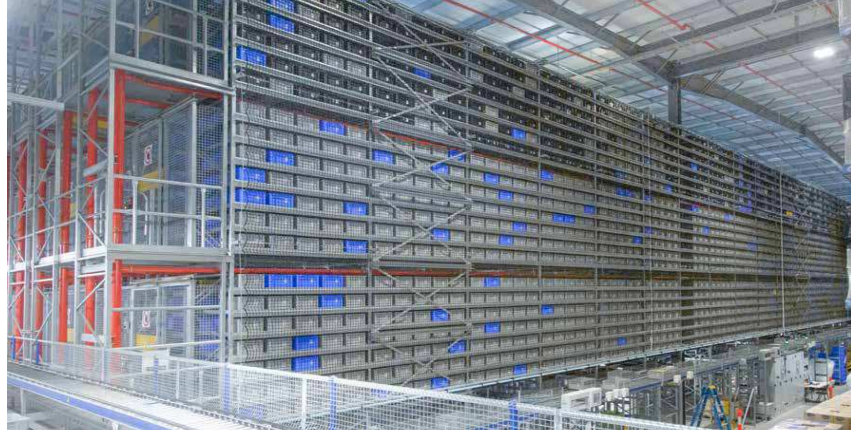
SSI Cuby shuttle system in the patented 3D-MATRIX configuration
