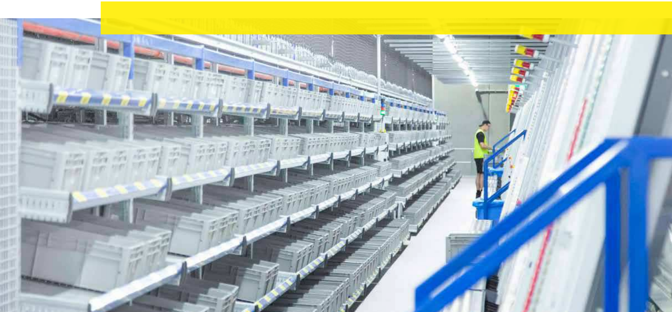
Carton live storage automatically replenished from the single-level shuttle system SSI CUBY arranged in the patented 3D MATRIX Solution® concept
