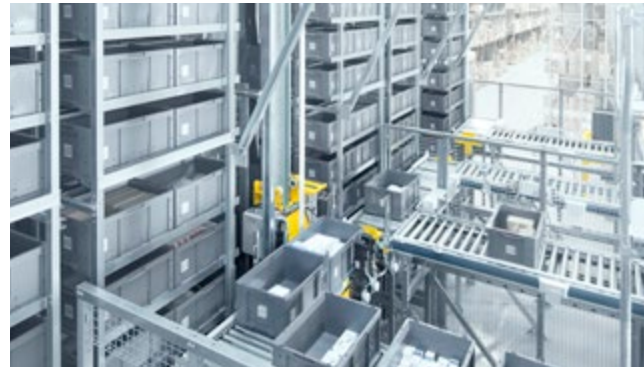
2 SEMI- AND FULLY AUTOMATED MINILOAD SYSTEMS
