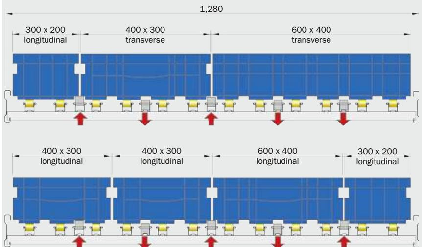
Retracting or extending the dividing rail enables containers with different dimensions to be mixed on one level
