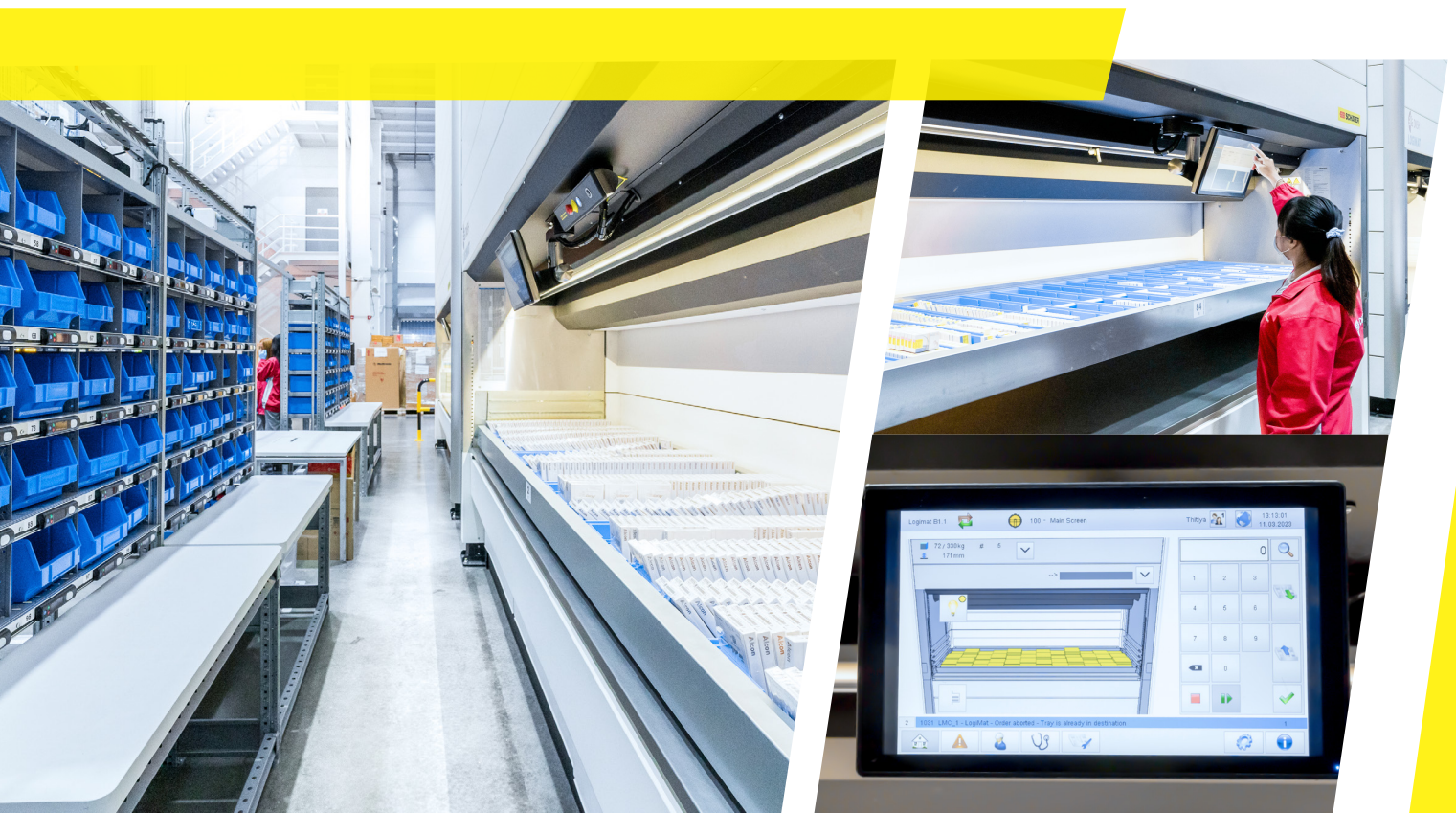
Small and loose SKUs such as surgical contact lenses are stored in the SSI LOGIMAT®
