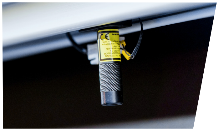
LogiPointer guides the picker to the correct SKU
