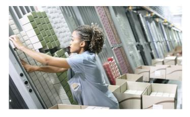
The A-Frame from SSI SCHAEFER performs complex order consolidations automatically, reliably, and as quickly as possible. It is particularly suitable for picking small packaging units without errors. Thanks to a sophisticated system with both straight and inclined product channels, the throughput of fast and medium movers is increased dramatically.
