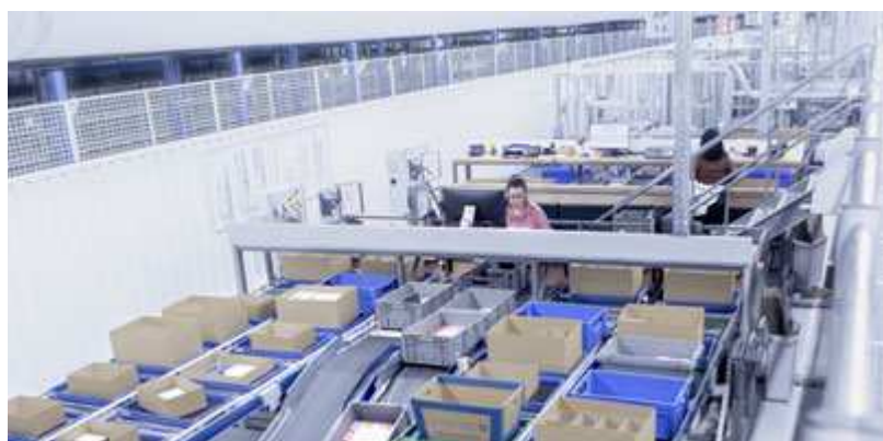
Advanced Pick Station one-level: picking of as many as four orders simultaneously at a single work station
