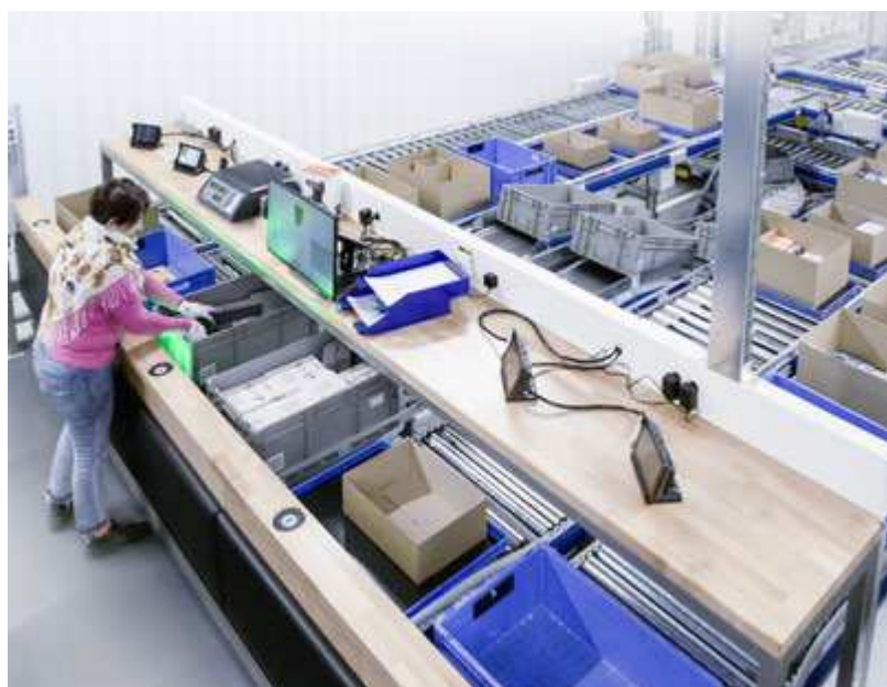
One-stop-pick solution: complete order picking at a single work station
