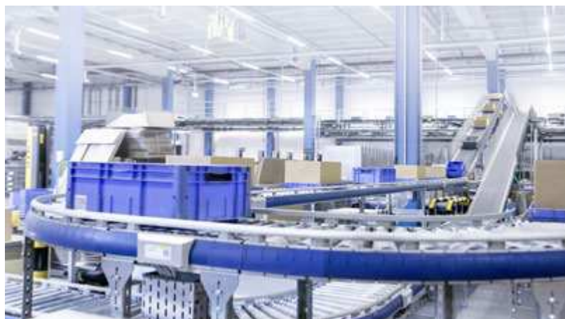
Transport of the order container or carton to the predetermined picking area
