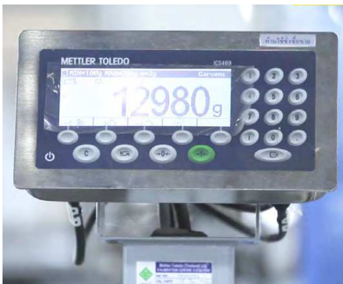
WAMAS® in direct communication with weight check stations
