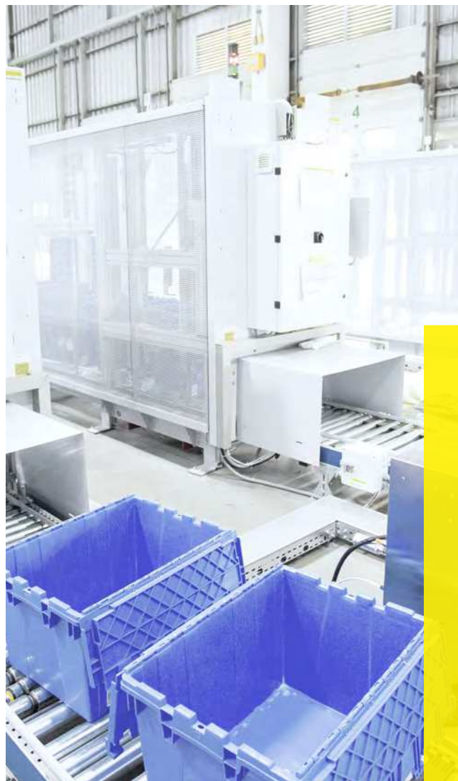
Destacking: 800 bins per hour / machine
