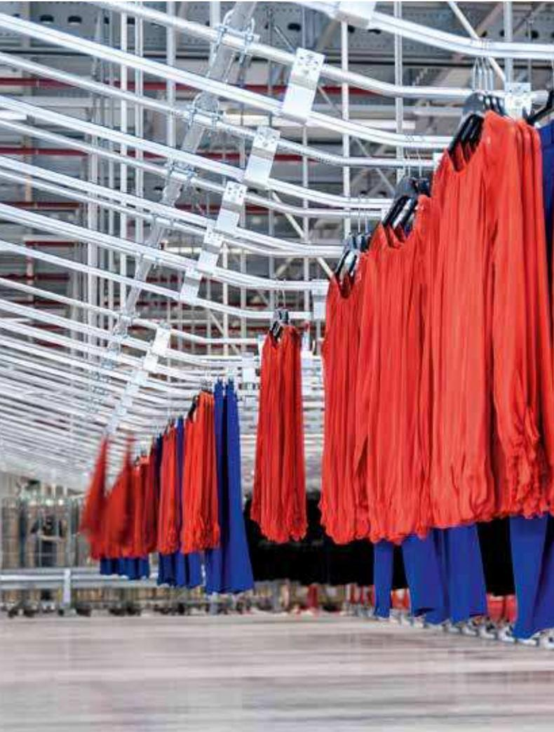
▼ Clip conveyor – accumulation function when clip is open
