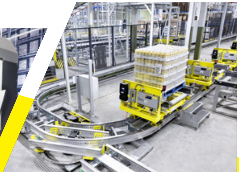
Transport to depalletizing via rail-guided vehicle system
