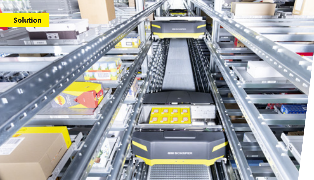
Storage and retrieval by SSI Flexi Shuttles
