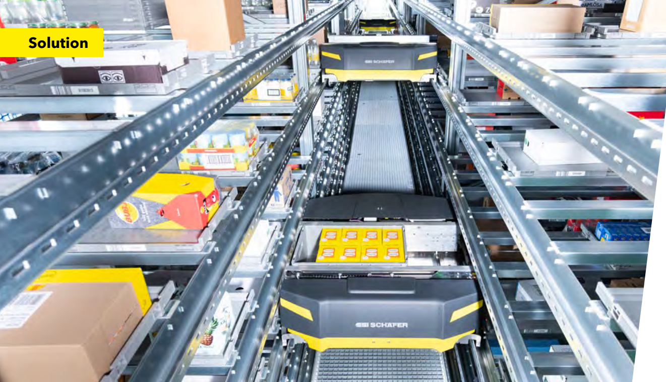
Storage and retrieval by SSI Flexi Shuttles
