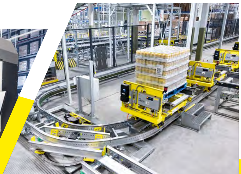
Transport to depalletizing via rail-guided vehicle system
