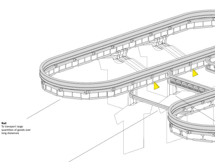
Push rail system For manual process steps such as quality check, labeling or putting garments on hangers; or as head of sorter
