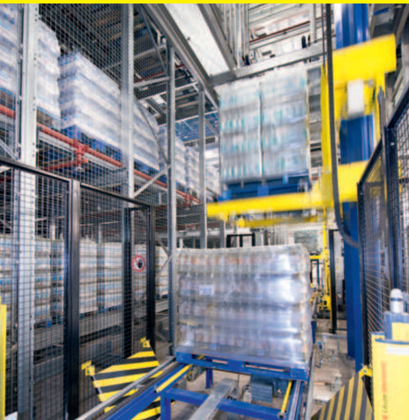
Picture above: The channel vehicle Schaefer Orbiter System (SOS) handles storages and retrievals
