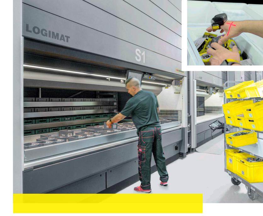
The vertical lift modules are controlled using a touch screen with a user-friendly and language-independent user interface that visualizes the information using icons, meaning no costly training period is necessary. Information displayed includes the device status and the items required for picking.
