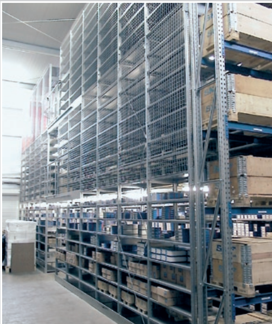
Storage mezzanine with rear grilles in Goods IN section, with pallet shelf to provide buffer storage
