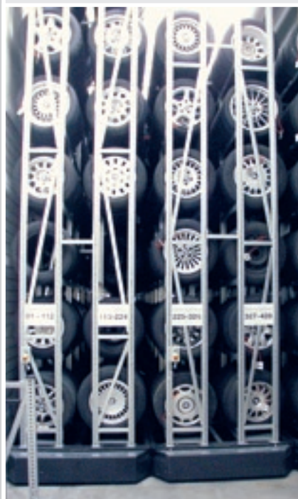
Electrically actuated heavy-duty sliding system, length 22 m – extendible and flexible
