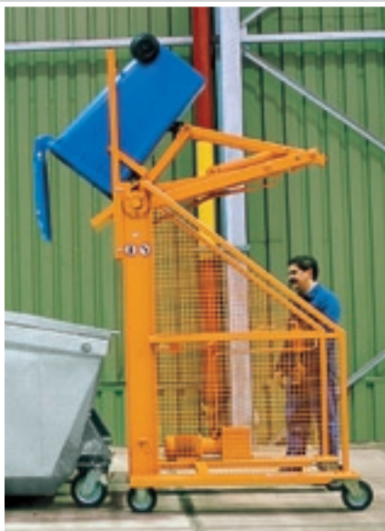
Automatic container tipper: for the easy handling of large refuse containers
