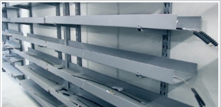
Horizontal storage of brake cables in cantilever-type shelf
