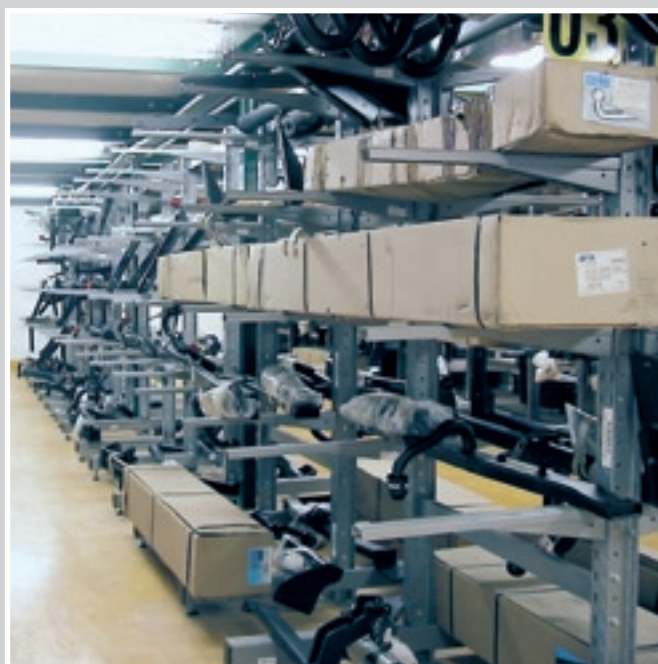
Storage of extra-long components in cantilever-type shelf
