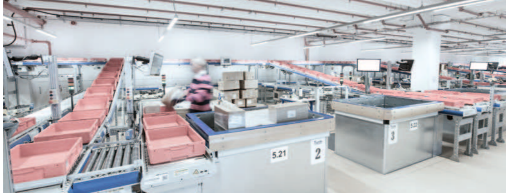
Manual scanning and repacking from pallets onto trays and into bins
