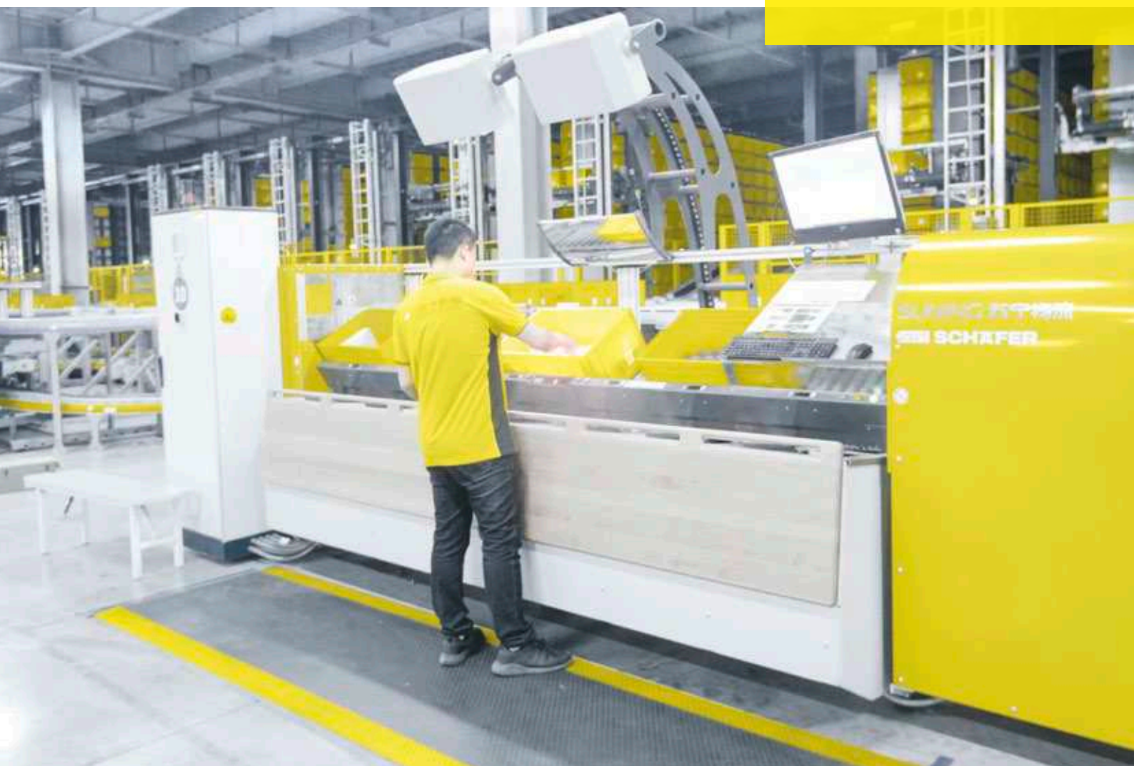
The "ergonomics@work!®" concept reduces bodily stress by moving loads only horizontally or by gravity
