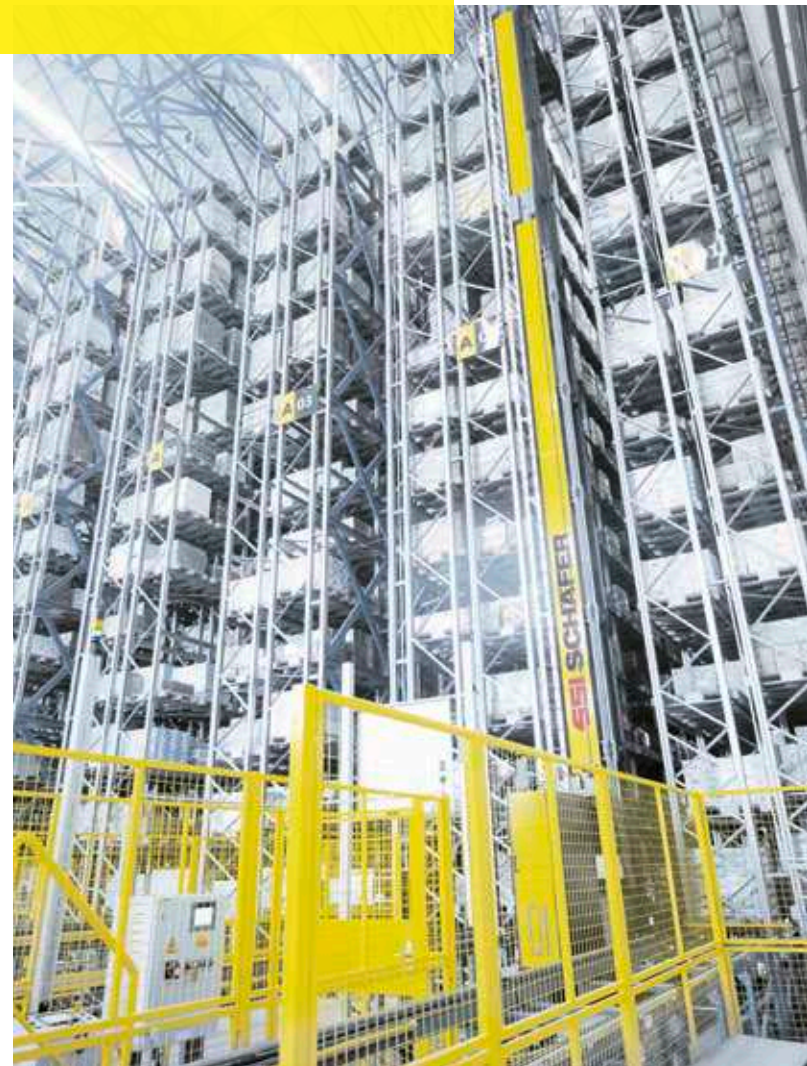
In the high-bay warehouse energy-efficient Exyz, modern pallet storage and retrieval machines, optimize the vertical warehouse space
