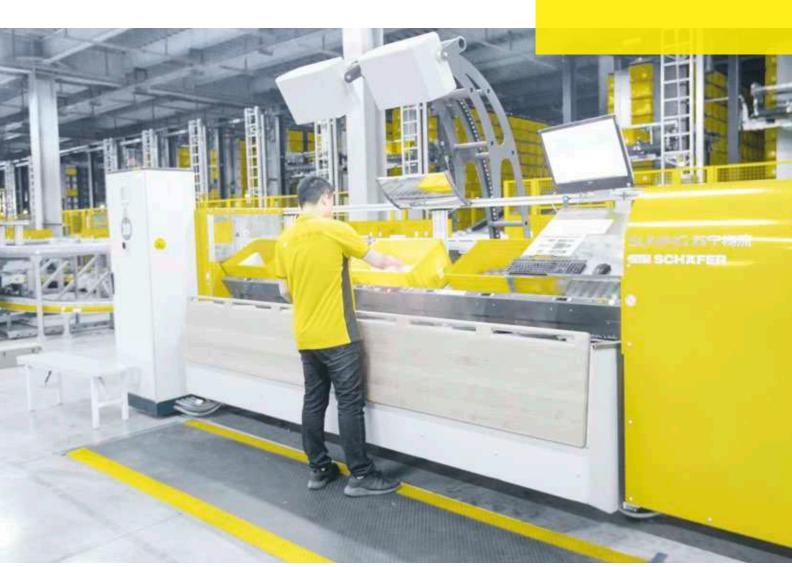
The "ergonomics@work!®" concept reduces bodily stress by moving loads only horizontally or by gravity
