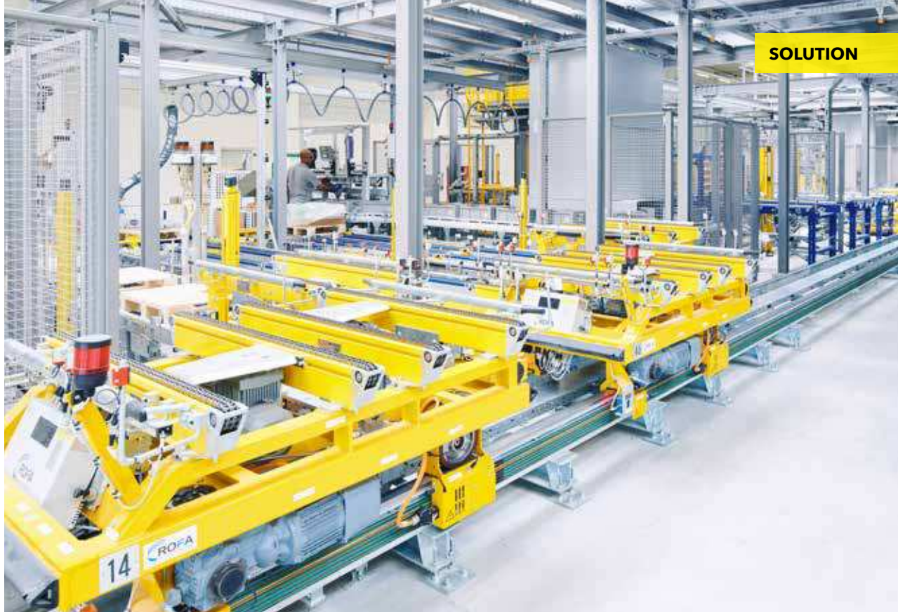
Pallet transport via electric rail-guided vehicle system
