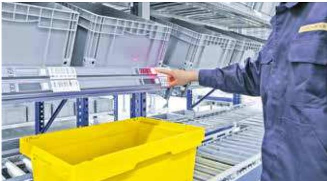
Pick by Light minimizes the number of picking errors. Each storage compartment is equipped with a signal lamp with a display and at least one acknowledgment button. If the order bin is placed in picking position, the lamp shows the employee the correct compartment, and the number of products to be picked appears on the display. Removal is then confirmed by pressing the acknowledgment button.
