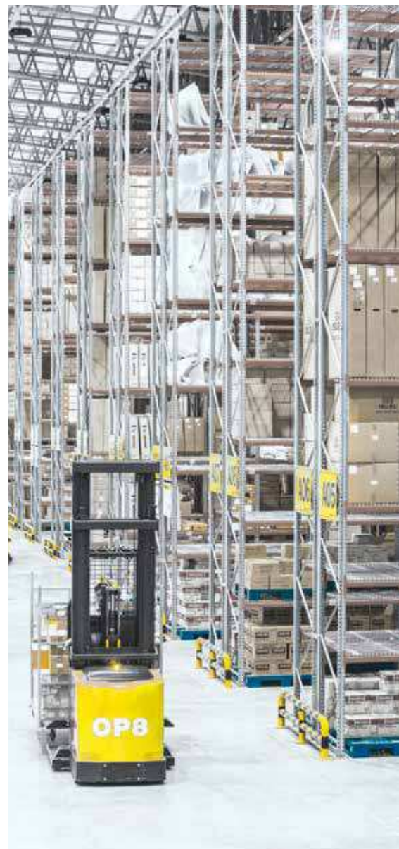
Selective pallet racking with 4,656 pallet locations
