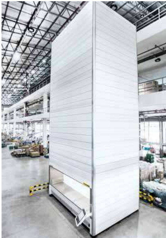
Vertical lift module SSI LOGIMAT® with 2,500 box locations
