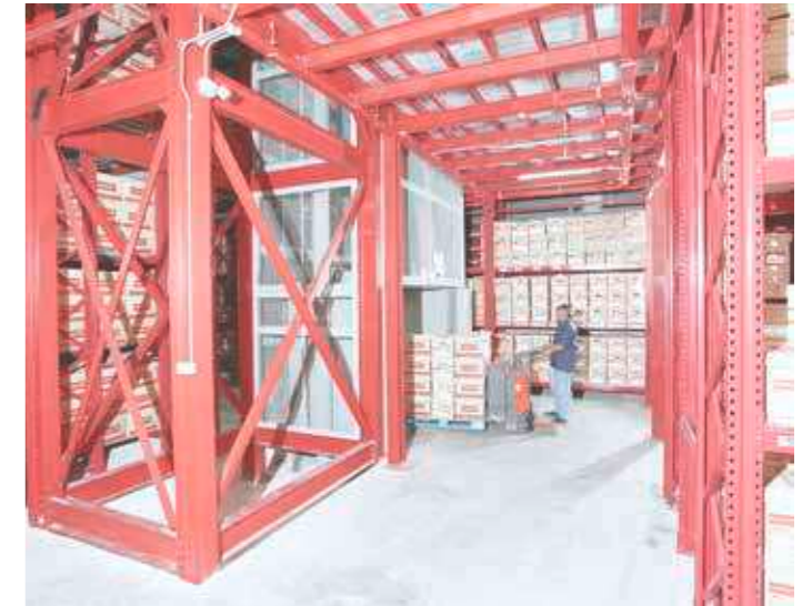
Goods lifting hoist for economic and more efficient cargo transfer between floors
